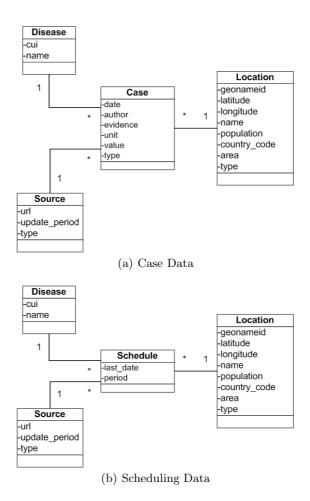
Fig. 3. UML class diagram of the MEDCollector Repository.
